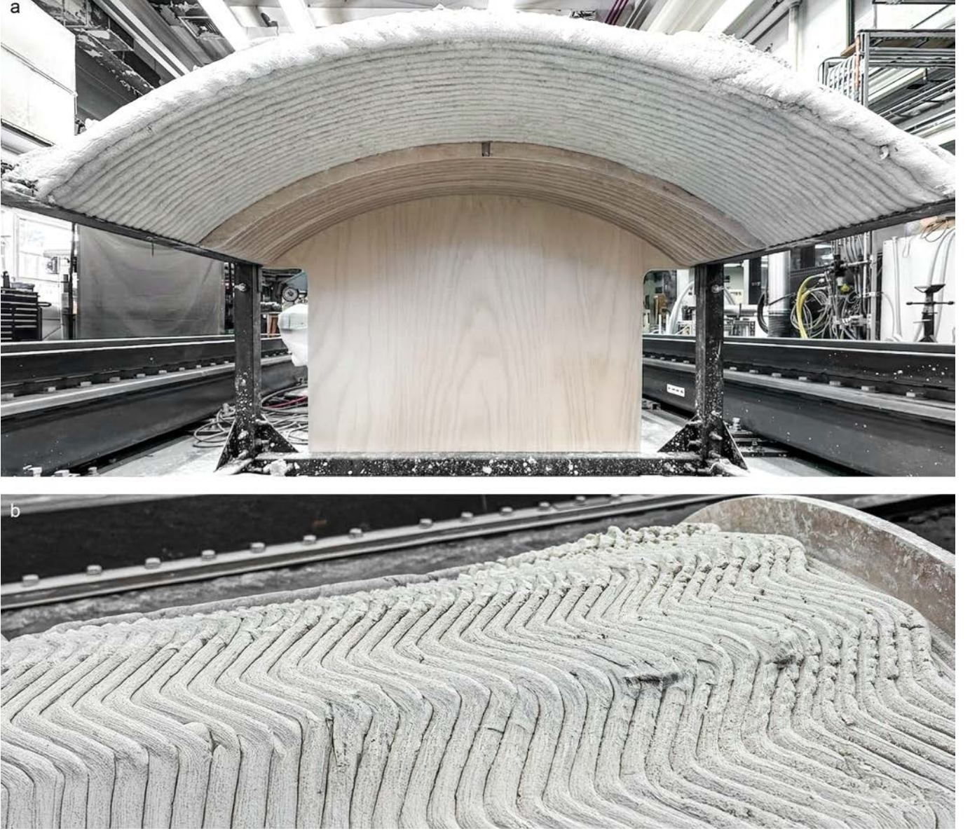
Figure 17: Experiment B: full barrel-vault print with (n_r, d_r) = (7, 4) at N_c = 1 . (a) Photograph during deposition: the primary filament and zig-zag lamination pass are visible; I_0 advances by p_p = 14 mm after each completed cycle. (b) Top-view photograph of the zig-zag pattern on the vault surface.
