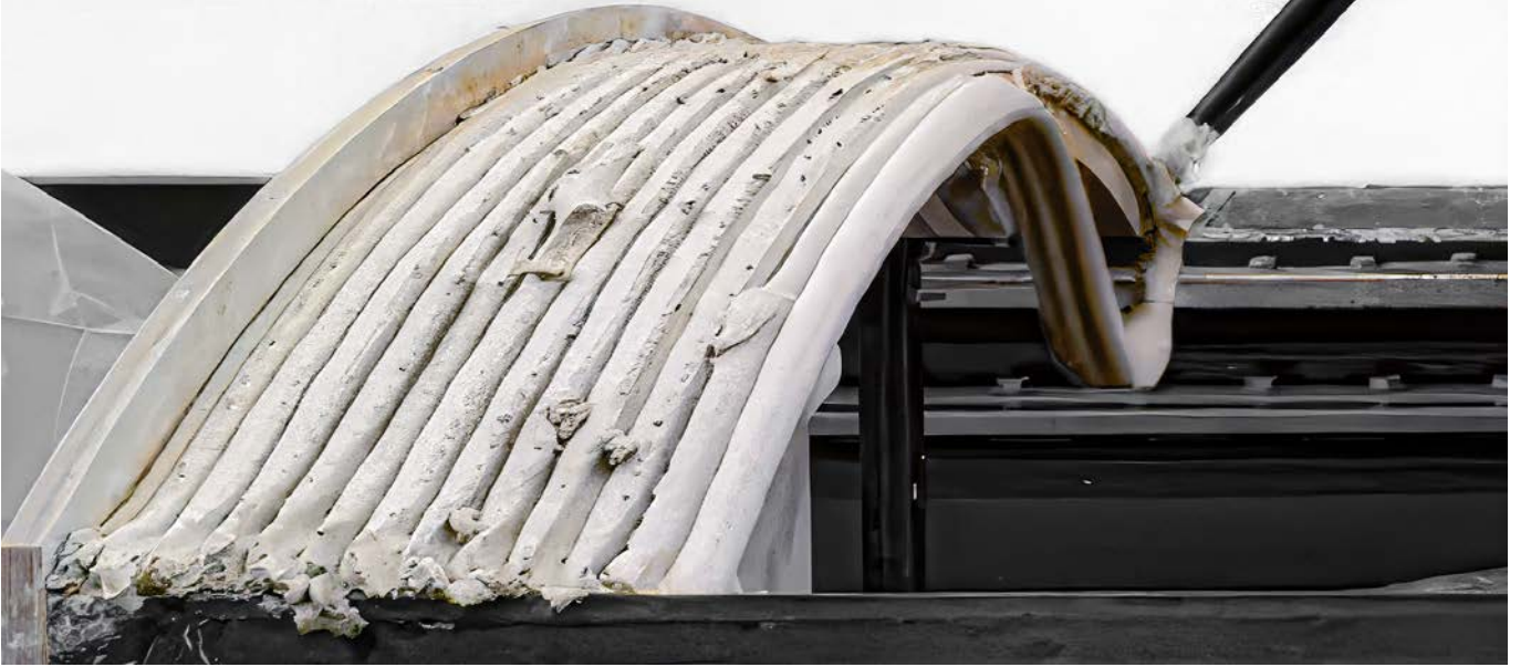
Figure 10: Experiment A: primary-only benchmark. The vault is printed without lamination; the cantilevering filaments beyond I_0^{(0)} delaminate at D = 42 mm ( N_c^{\text{crit}} = 3 filaments), peeling away from the root interface under their own weight.
