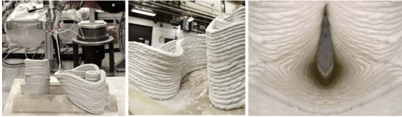
Fig. 6. View of the printed optimized beam segment showing consistent layer height and width across multiple areas, along with noticeable deformation in certain regions.
