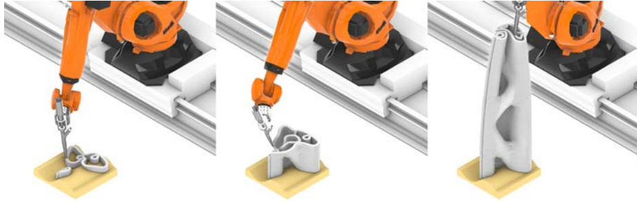
Fig. 3. Experimental validation of the proposed motion-planning framework on a topology-optimized branched beam. The complex geometric features make it a representative case for studying the coupled requirements of time-dependent orientation feasibility and volumetric accuracy.
