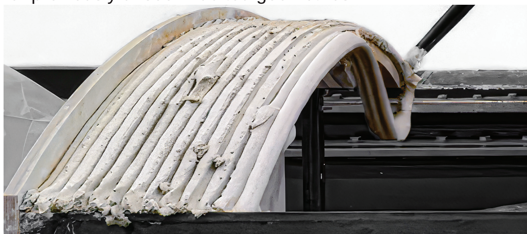
Figure 2: Primary-only benchmark (Experiment A). Without lamination, cantilevering filaments peel away from the root interface under self-weight after only 3 filaments (42 mm), demonstrating the fundamental cantilever limit of single-layer 3DCP.
