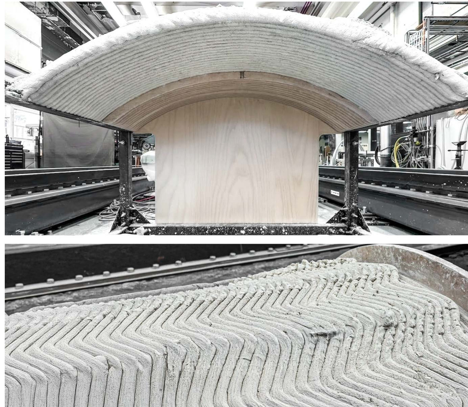
Figure 6: Experiment B: scaffold-free barrel vault printed with the selected lamination design. (Top) Completed vault during printing, showing primary filaments and zig-zag lamination passes. (Bottom) Top view of the zig-zag pattern on the vault surface.
