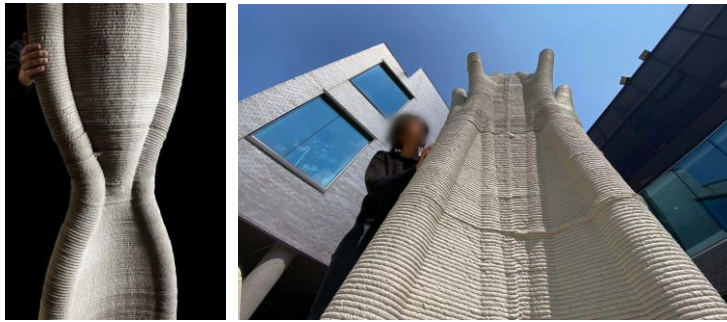
Fig. 6 3D concrete printed topology-optimized walls: Shell Wall (left) and Branch Wall (right)
