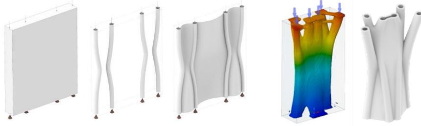
Fig. 2 Topology optimization process and geometric post-processing: Shell Wall (left) and Branch Wall (right)
