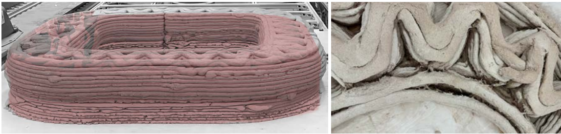
Figure 10: Left image: Deformation resulting from the plastic failure in the prototype printed through the R-3DP, Right image: Demonstrates the delamination of the object manufactured using the MR-3DP process using material (F2). Source: (Created by the authors 2024)
