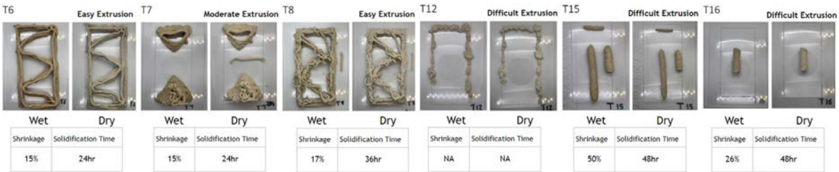
Figure 2: Different material compositions employed in experiments for material research. Source: (Created by the authors.)
