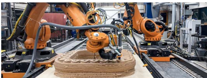
Figure 9: Resulting construction scale prototype from the R-3DP process with wood-based slurry material using material (F1). Source: (Created by the authors 2024)
