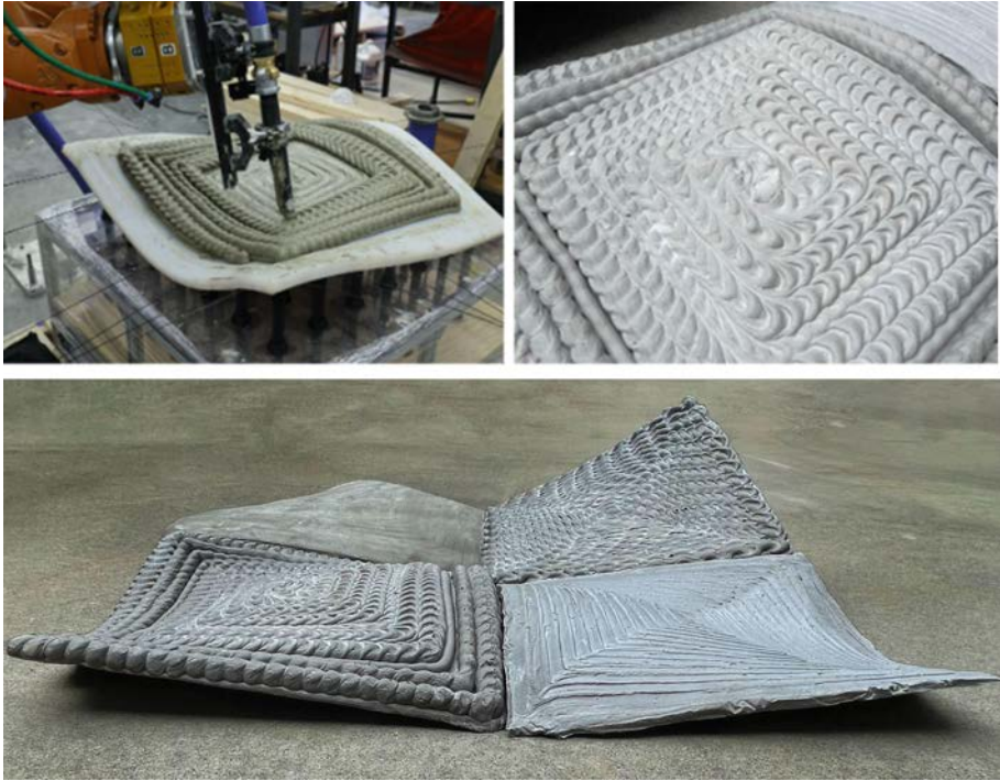
Fig. 6. Resulting freeform panels from the developed process.
