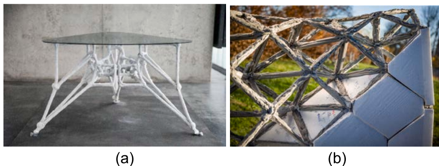
Fig. 12. Examples of 3D printing on temporary supports: a) Case study fabricated table presented by Xiao et al. [64] the legs of the table were optimized using Vector-based 3D Graphic Statics and 3D printed in a limestone-based carrier liquid, b) Space truss 3D printed on EPS foam blocks presented by Duballet et al. [65].
