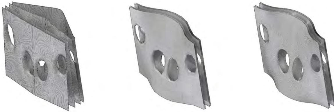
8 Left is the resulting minimal surface with two topology regions and their interconnecting channels derived from the SGAMS algorithm. The middle a parametric adaptation of the topology to the functions and reconstruction of the minimal surface with rough mesh faces. Right is an increase in the mesh faces to increase surface resolution.
