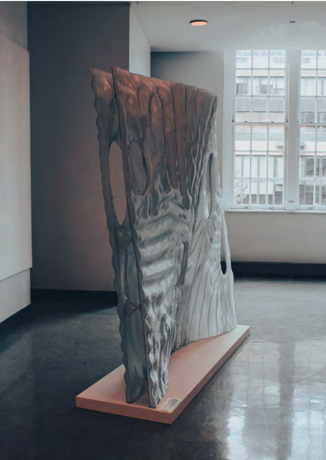
11 The 1:1 scale prototype is made of two thermoplastic elements.
