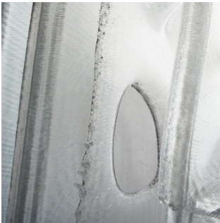
9 Fabrication images of the full-scale prototype highlighting the seamless connection of channels and interior layers.
