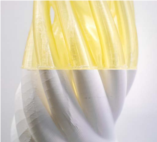
10 Matrix detailing the material, print setup, and formwork geometry developed through prototyping, which allows for successful 3D printing of formworks and cross-referencing between different formwork systems. 11 Intersection of PLA and PVA materials on a case study column formwork.
