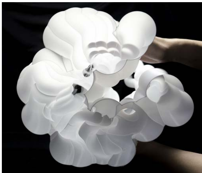
3 Ultrathin 3D printed PLA formwork with a 0.8 mm wall thickness.
