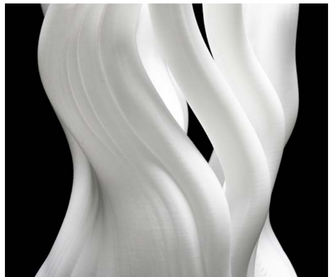
4 Detail of the layer resolution used for ultrathin 3D printed PLA formwork.
