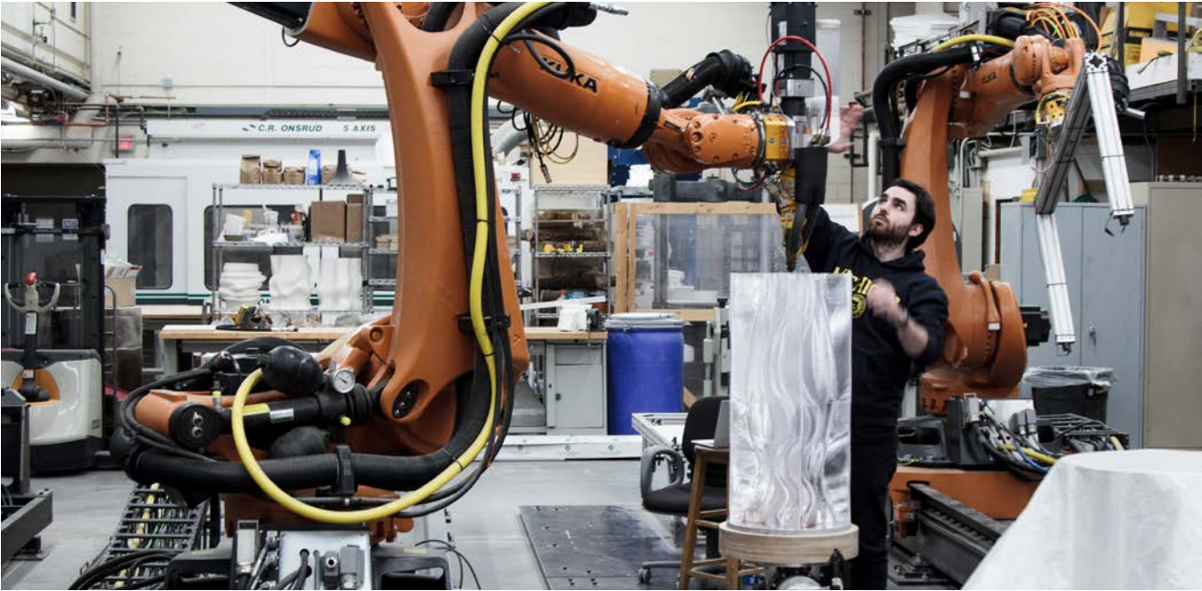
2 Robotic arm fitted with a custom-fabricated pellet extrusion end-effector.
