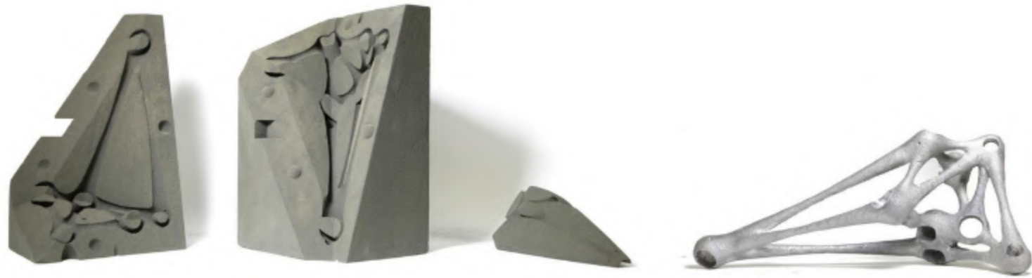
Figure 4. A 3D printed sand mold (left) and an aluminum cast joint (right), the MAS DFAB at ETH Zurich 2017. Photographer: Ma Xije
