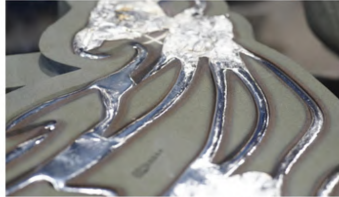
Figure 2. Cast metal in 3D-printed sand-molds
