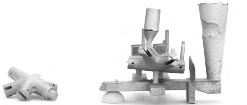
Figure 4. The image shows a FDM-printed of a joint design (left) and the final cast joint before post-processing (right). The gating system needs to be removed from the joint, thus the articulation of the interface is important. Photographer: Axel Crettenand.
