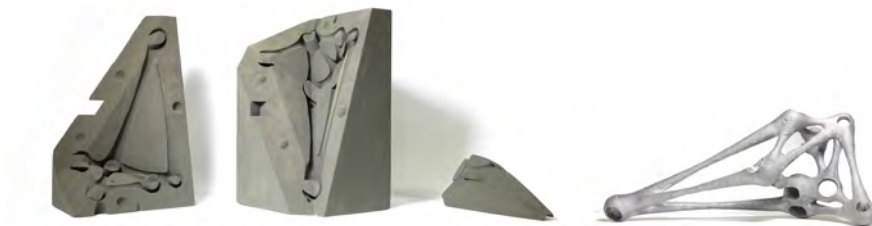
Figure 1. 3D printed segments of a sand mold and a cast aluminium node. Photographer: Ma Xije.
