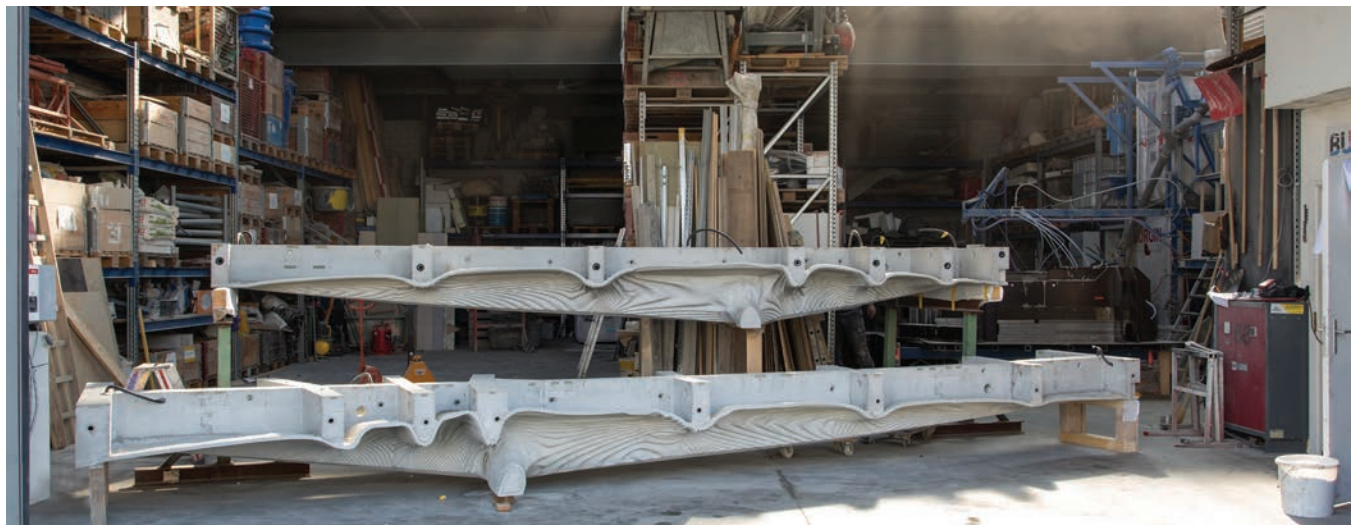
19 A prefabricated concrete segment made of sprayed 20-mm-thick fiber-reinforced concrete shell and cast upstand ribs above.
