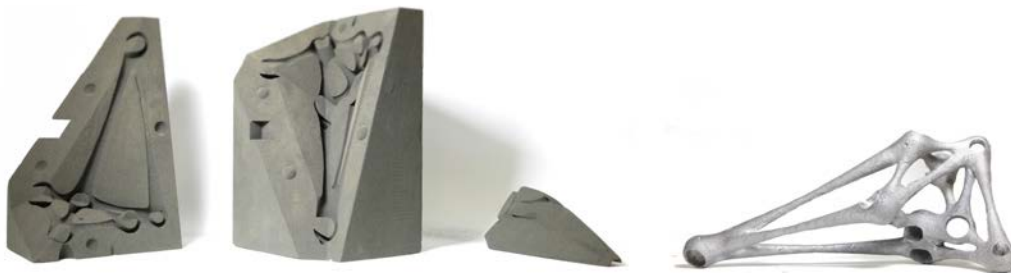
Figure 2: Segmented mold and cast node. Photographer: Ma Xije
