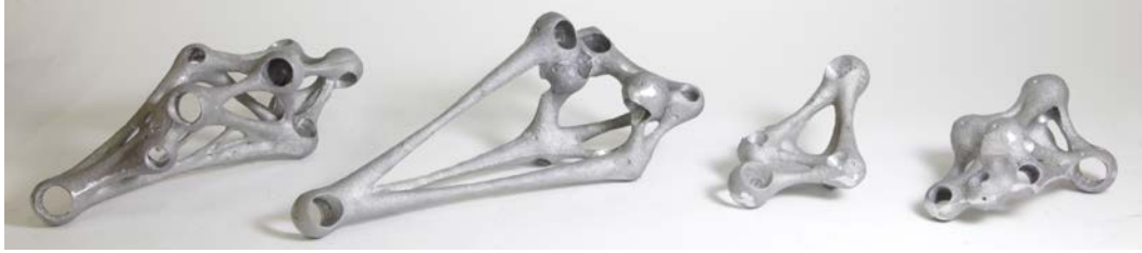
Figure 4: Variation of small sized parametric nodes. Photographer: Ma Xije
