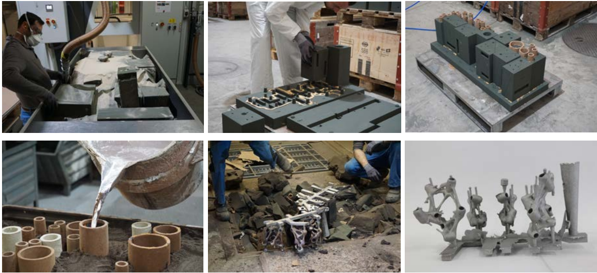
Figure 7: a) Unpacking of 3D printed sand molds, b) Assembly of multiple molds on a gating system c) 3D printed mold with casting systems, d) Casting process e) Demolding using vibration platform of gating system, f) an array of metal nodes with ingate system.
