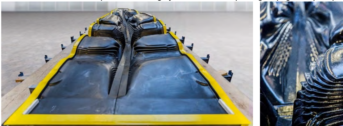
Fig. 8. 3D-printed formwork for a 7.1-m concrete slab segment (left) and close-up detail (right).
