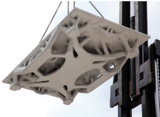
Figure 7, left. Prototype “B”; topology optimization of a slab with four supports.
