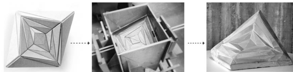
Figure 7: Folded MDF, Formwork setup, cast object. Design: Gusten Eriksson Hemström, Robin Lee, Maxime Boileau, Björn Liljeqvist
