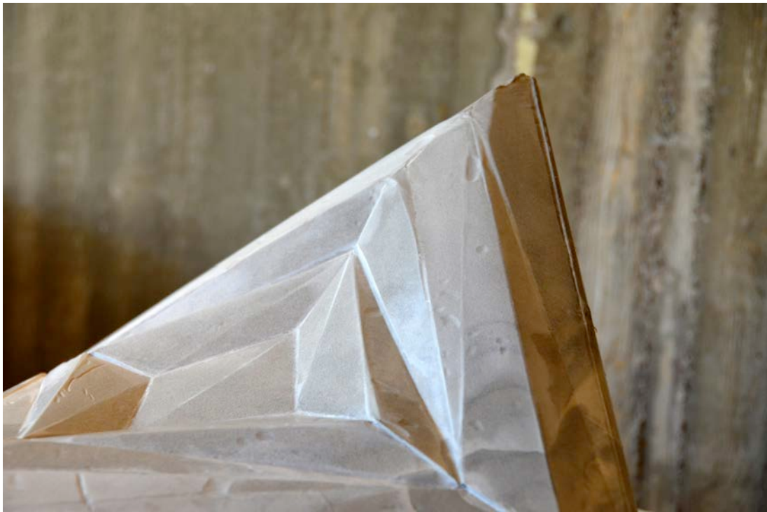
Figure 8: Concrete demonstrator object made with our hinging dynamic formwork system. Design: Gusten Eriksson Hemström, Robin Lee, Maxime Boileau, Björn Liljeqvist
