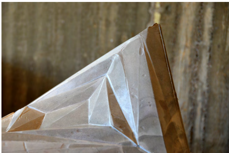
Fig.1 Concrete component casted from dynamic formwork.
