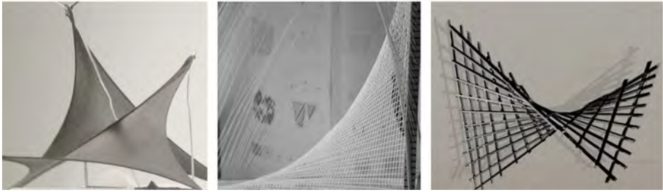
Fig. 3 Materializing the hypar with fabric, string network and wood rods.
