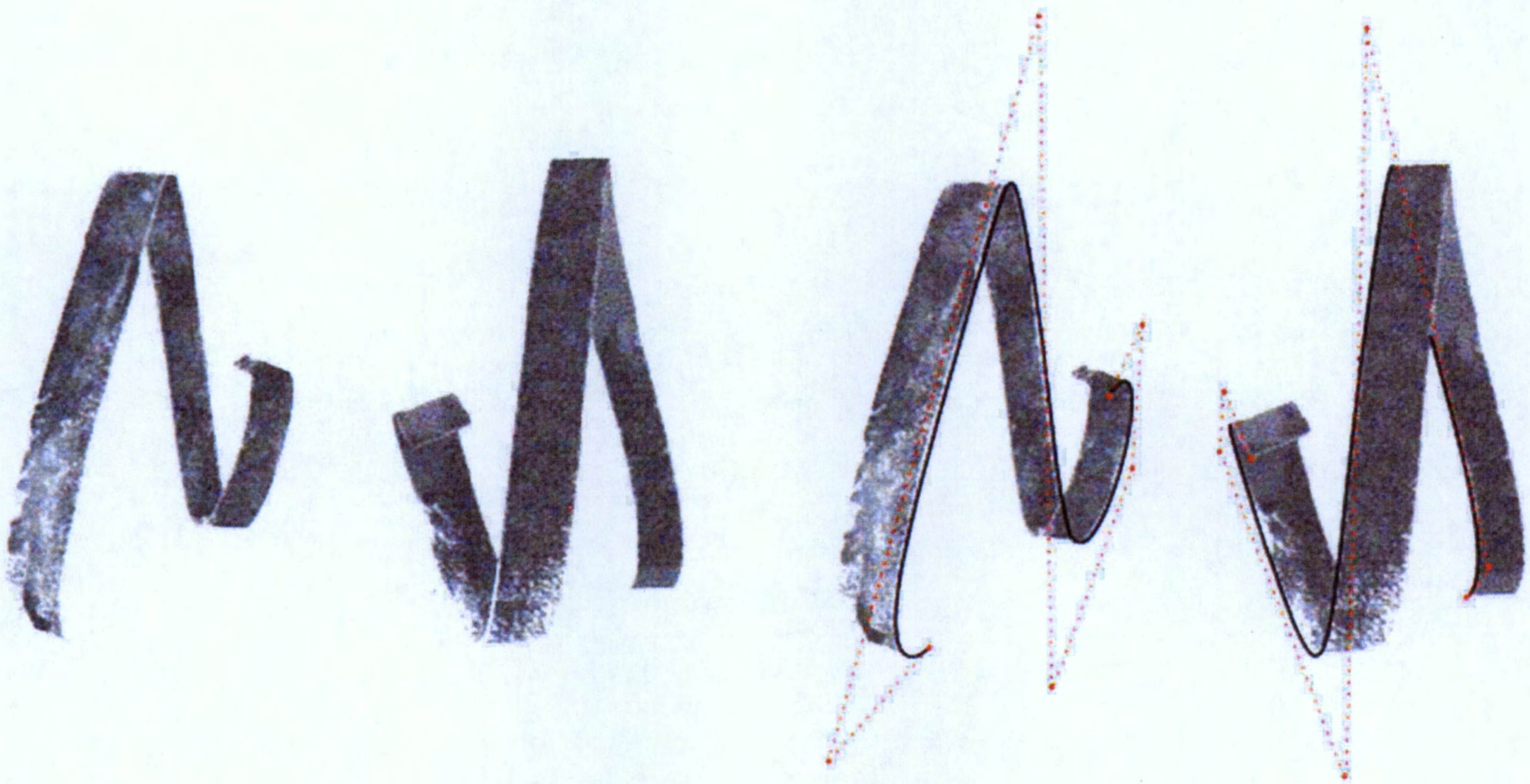
Fig. 5 Extraction of curves from point clouds of paper stripes.
