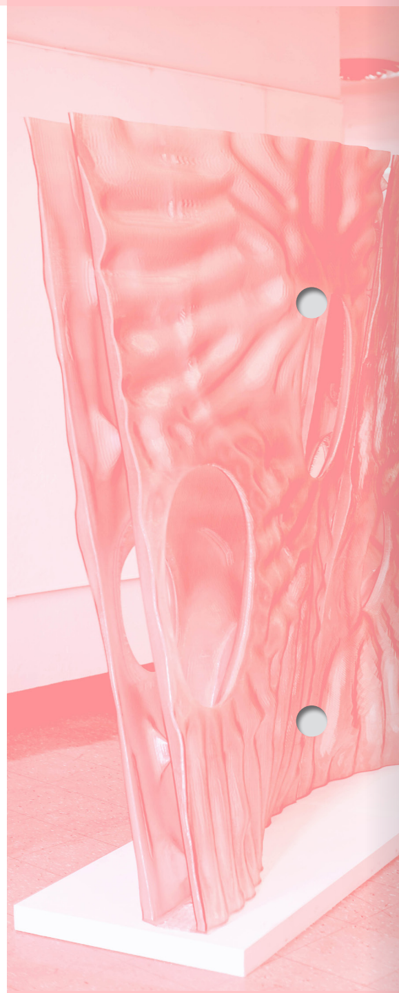
Robotic 3D printed multilayer building envelope (2.5 m high x 2.5 m wide) with complex topology and reaction-diffusion surface undulation
