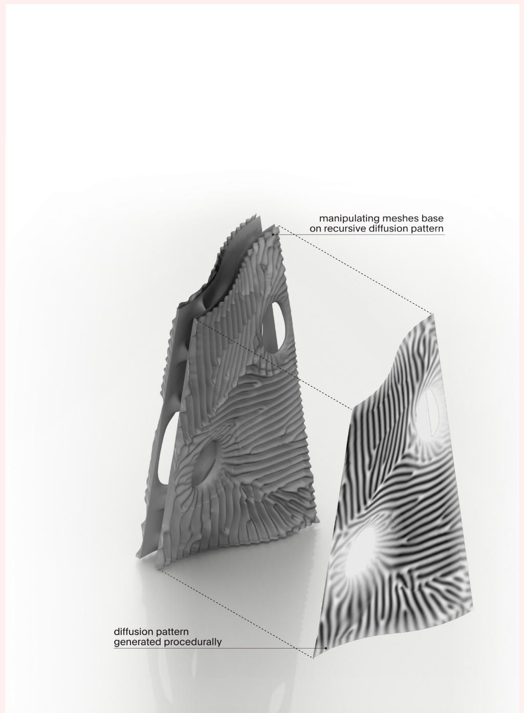
[Fig. 6] Reaction-diffusion pattern is adjusted in scale and mesh resolution is increased using Catmull-Clark methods.
