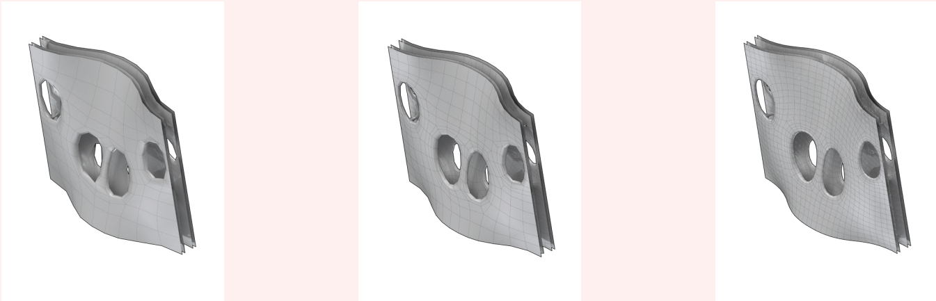
[Fig. 2] 3D model evolution of the multilayer building envelop through the articulation of the layer distances and mesh resolution
